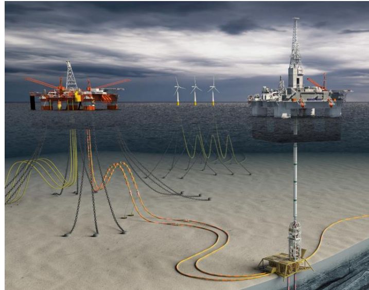
Figure 11-3: Pipeline in Subsea Area (Known as umbilical)
